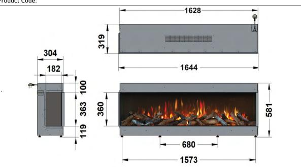
FRAME BUILD OUT DIMENSIONS (All dimensions are in millimetres)
