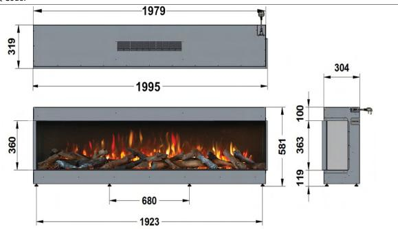
FRAME BUILD OUT DIMENSIONS (All dimensions are in millimetres)
