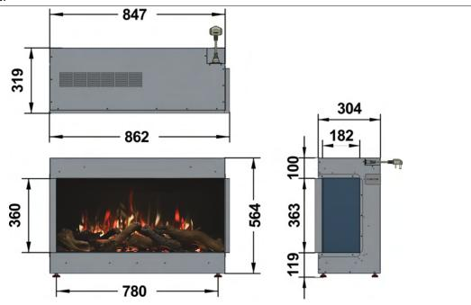
FRAME BUILD OUT DIMENSIONS (All dimensions are in millimetres)
