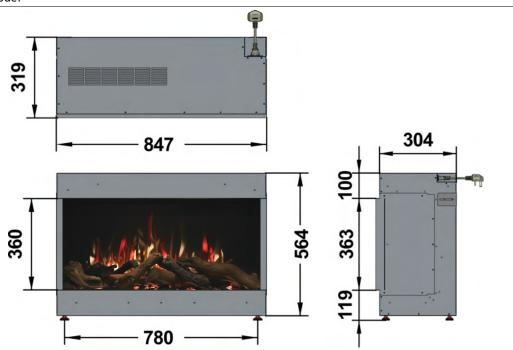
FRAME BUILD OUT DIMENSIONS (All dimensions are in millimetres)
