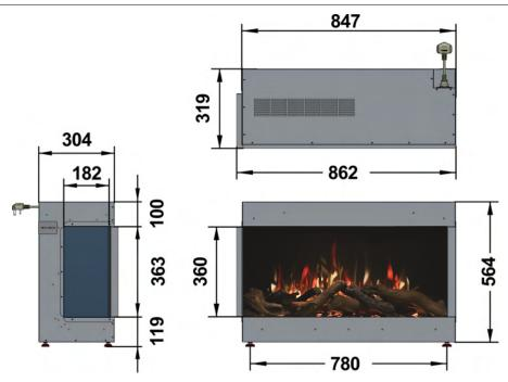
FRAME BUILD OUT DIMENSIONS (All dimensions are in millimetres)
