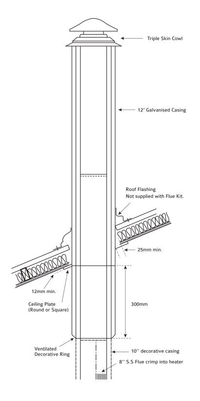
If the appliance is connected to a masonry chimney, it is recommended a chimney register be installed above any installation into a masonry fireplace minimizing heat loss up the chimney.
