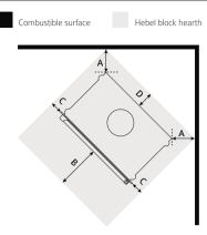
Protector Board - 50mm Skamol or 60mm Calcium Silicate board or 75mm Hebel
