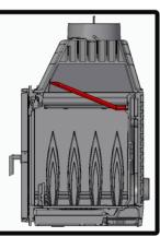
Position of the baffle from side view
