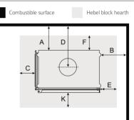
$\square$ Protector Board - 50mm Skamol or 60mm Calcium Silicate board or 75mm Hebel
