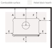
Protector Board - 50mm Skamol or 60mm Calcium Silicate board or 75mm Hebel
