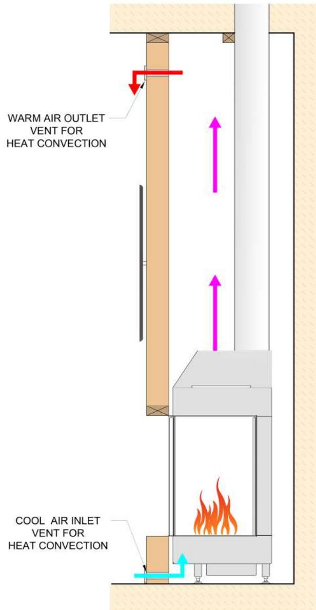
Figure 1.1 (Convective heat through vents)
