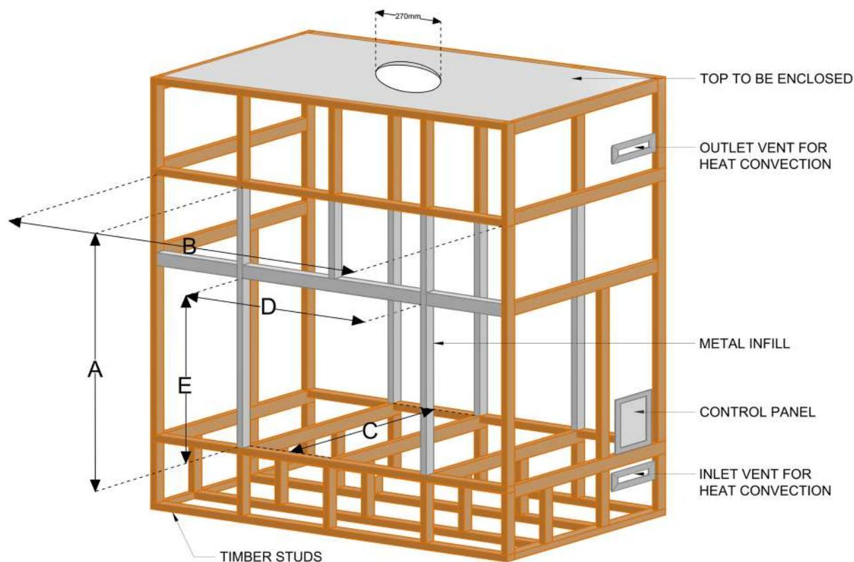
Figure 1.8 (Timber framing)
